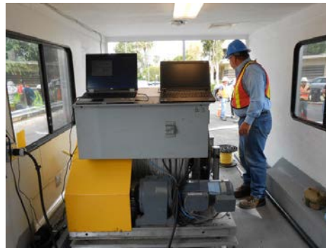
The location of the NDE tool is tracked by measuring the amount and speed of tether rope deployment. Underneath the table is the motor used to winch back the tool. All tools and equipment were powered from a small electrical generator.
