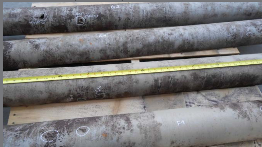
Uncorroded pipe measurements were generally 7/16-inch thickness (0.43 inch).
