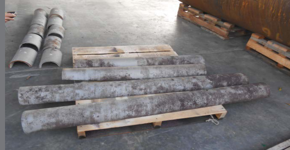
Seven pipe segments were split longitudinally into 14 pieces, then sandblasted.
