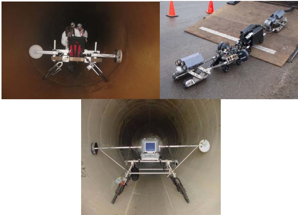
Figure 3-10. P-Wave ® System for Manned and Robotic PCCP Inspection (Reprinted with permission from Pure Technologies)
