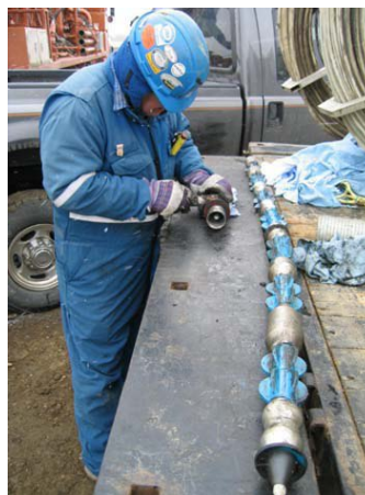
Figure 3-9. The See Snake Tool for Inspection of Pipe Internal and External Flaws (Reprinted with permission from Russell NDE Systems Inc.)
