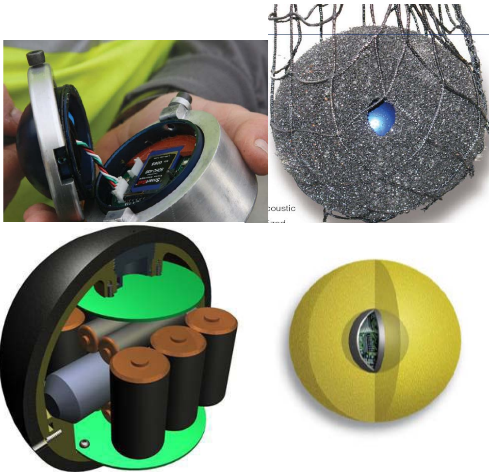
Figure 3-12. Pictures and Illustrations of SmartBall®: internal view (left) and external view (right) (Reprinted with permission from Pure Technologies)
