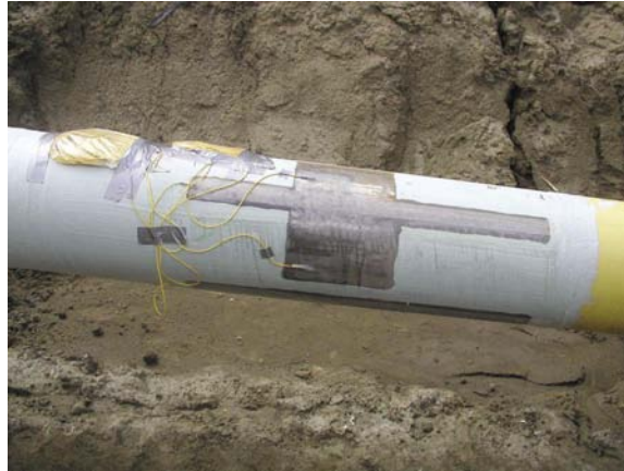
Figure 3-28. Monitoring Corrosion and Bending of Pipelines with Fiber Optic Sensors (Reprinted with permission from FOX-TEK)
